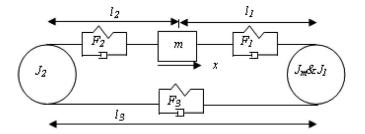
Fig. 4. Physical model of the linear servo drive.
