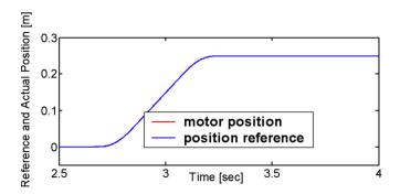
Fig. 5. Position tracking of the motor.
