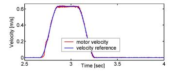
Fig. 7. Velocity tracking of the motor.
