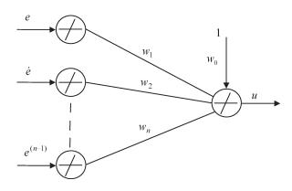
Fig. 2. Structure of the NN for SISO systems.
