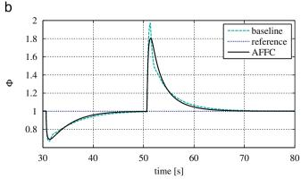
**Fig. 5.** Comparison of baseline controller and AFFC: (a) response to a set-point change and (b) response to purge disturbance (simulation).
