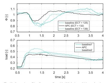
**Fig. 10.** Comparison of baseline controller with APC during vehicle acceleration, with c=1.5. ECT stands for engine coolant temperature (experiment).
