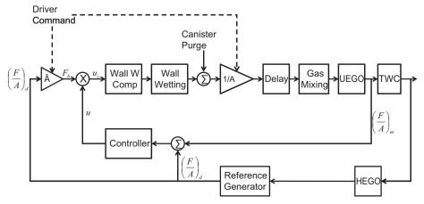
Fig. 2. Overall closed loop controller structure.
