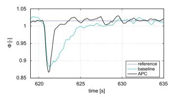
**Fig. 8.** Comparison of baseline controller with APC for purge disturbance rejection at  $1000 \, \text{rpm}$ , with c = 1 (experiment).
