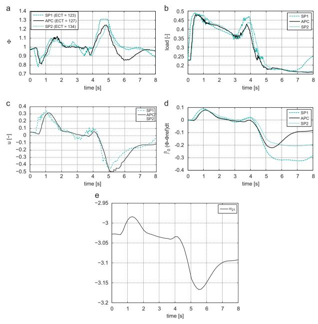
Fig. 11. Time histories of: (a)  $\Phi$  (ECT stands for engine coolant temperature), (b) engine relative air flow, (c) feedback control input, (d) tracking error integral, during vehicle acceleration and deceleration for gain-scheduled SP vs. APC, with c=1.5, and (e) evolution of the first component of  $\alpha_2$  (experiment).
