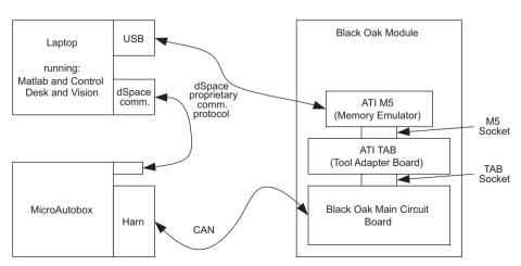
Fig. 4. Rapid prototyping with MicroAutobox using CAN.
