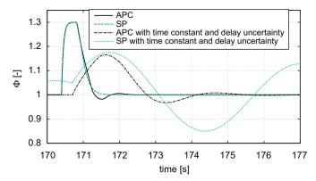
**Fig. 13.** Comparison of SP and APC for input step disturbance rejection in the presence of sensor time constant and delay uncertainty (simulation).
