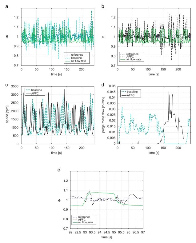
**Fig. 6.** Baseline controller vs. AFFC: (a)  $\Phi$  and air flow rate when baseline controller is active; (b)  $\Phi$  and air flow rate when AFFC is active; (c) engine speeds; (d) purge fuel flow rates; and (e) 5-s window zoomed from subfigure (b) (experiment).
