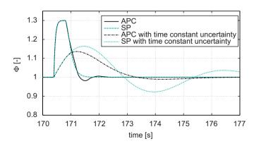
**Fig. 12.** Comparison of SP and APC for input step disturbance rejection in the presence of sensor time constant uncertainty (simulation).
