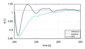
**Fig. 7.** Comparison of baseline controller with APC for purge disturbance rejection at 700 rpm (experiment).
