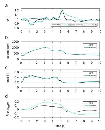
**Fig. 9.** Time histories of: (a)  $\Phi$ , (b) engine speed, (c) engine relative air flow, (d) tracking error integral, during vehicle acceleration and deceleration for APC vs. baseline controller, with c=1 (experiment).
