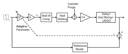
Fig. 3. Inner-loop structure with AFFC.
